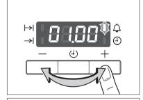
After approx. 5 seconds the display shows the time remaining. The function indicator Countdown △ lights up.
